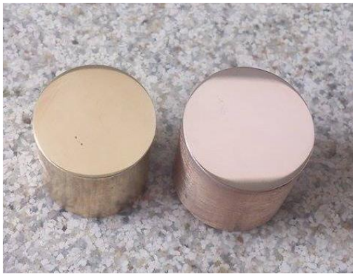
FIGURE 1: TEST TUBES ANALYZED THE TEST TUBE OF THE LEFT IS OF BRASS 60-40 AND THE TEST TUBE OF THE RIGHT IS BRONZE SAE 64. AUTHORS 2015
