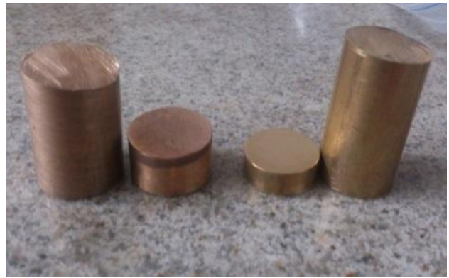
FIGURE 2: MATERIAL IN STATE OF DELIVERY, IN THE STUDY, WAS EMPLOYED TEST TUBES OF 1" X 1 1/2". AUTHORS 2015
