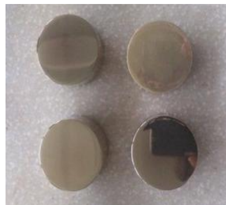
FIGURE 7: POLISHED TEST TUBE MIRROR SHINE BY MEANS OF SANDPAPERS FROM THE 80 UNTIL THE 1500 FOLLOWED OF CLOTH WITH OXIDE OF CHROMIUM. AUTHOR OF THE PROJECT 2015.
