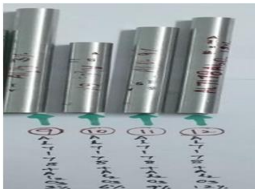
FIGURE 3: Machined Al7178 MMC's
