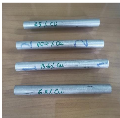
FIGURE 2: Al2021 Electrodes with varying % of Cu
