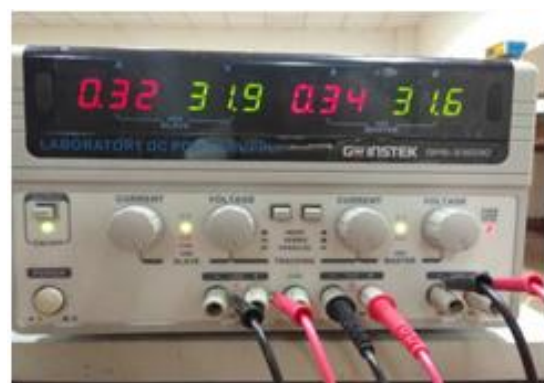
FIGURE 3: GUWEI DC POWER SUPPLY
