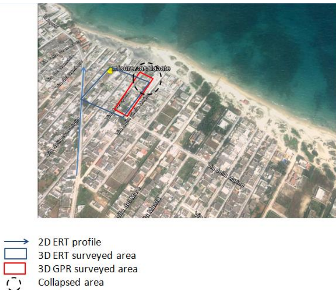
FIG. 3 – ERT AND GPR SURVEYED AREAS
