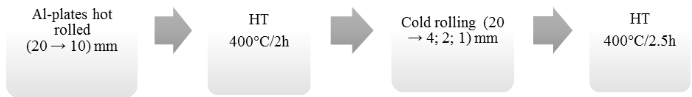
FIG. 2: AL-STRIPS PROCESSING (HT: HEAT TREATMENT, HR: HOT ROLLING)
