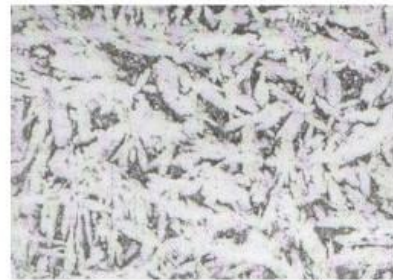
FIGURE 4. MICROSTRUCTURE OF ALLOY, HOT DEFORMED (x960)
