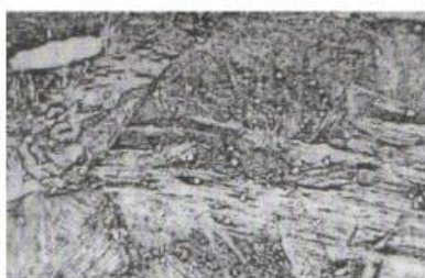
FIGURE 5. MICROSTRUCTURE OF ALLOY, ANNEALED AT 850 °C FOR 10 MIN AND WATER QUENCHED (x960)
