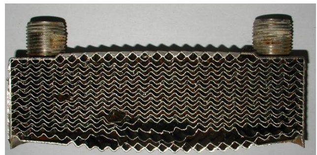
FIGURE 2: Deformation of the soldered joints of boards
