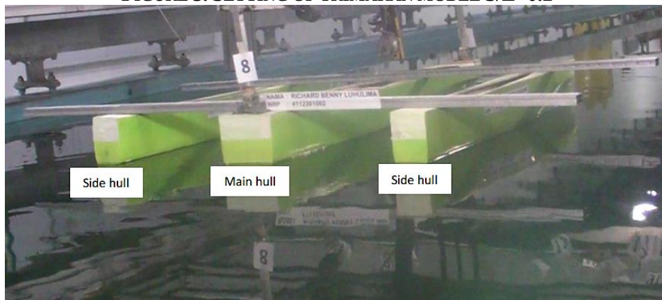
FIGURE 4. SETTING OF TRIMARAN MODEL S/L=0.3
