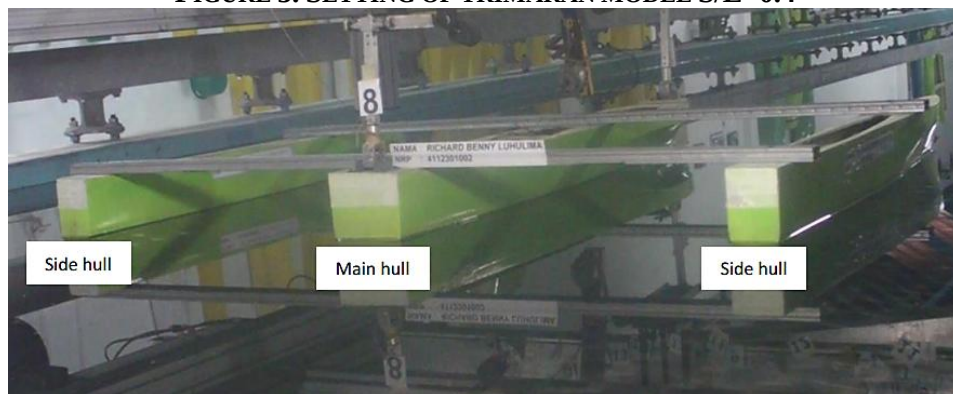
FIGURE 6. SETTING OF TRIMARAN MODEL S/L=0.5
