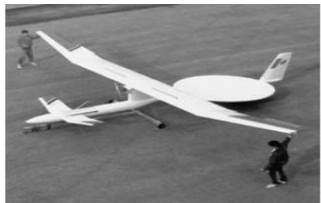
FIG.3: STATIONARY HIGH ALTITUDE RELAY PLATFORM.
