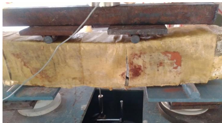
FIG 17 RETROFITTED SPECIMEN AFTER FAILURE
