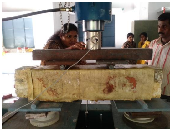
FIG 15 TESTING OF BEAM AFTER RETROFITTING USING GFRP
