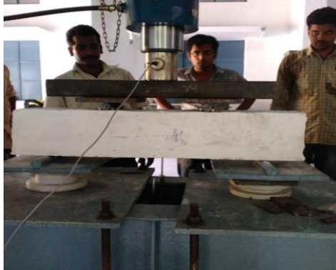
FIG 13 CRACKING OF BEAM BEFORE RETROFITTING
