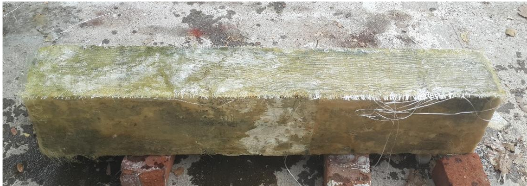
FIG 10 GFRP WRAPPING ON THE BEAM
