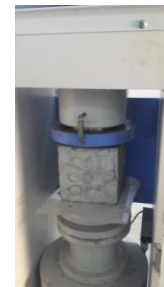
FIG 9 COMPRESSION TEST FOR THE CUBE ON 7 DAYS CURING
