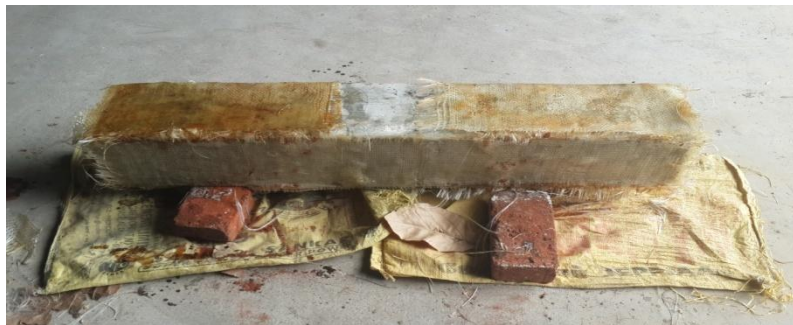
FIG 15 BINDING OF WOVEN MAT OVER THE GFRP SHEETS
