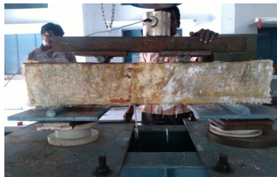
FIG 16 TESTING OF BEAM AFTER STRENGTHENING
