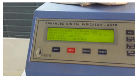
FIG 9 COMPRESSION TEST FOR THE CUBE ON 7 DAYS CURING
