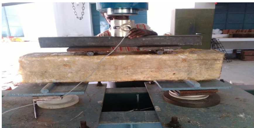
FIG 18 TESTING OF FULLY WRAPPED BEAM
