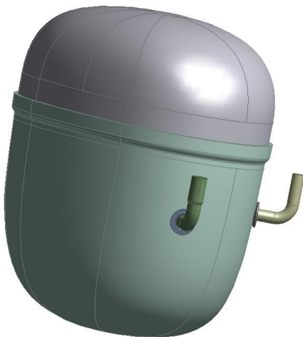
FIG. 5 REDUCED GEOMETRY OF THE COMPLETE COMPRESSOR
