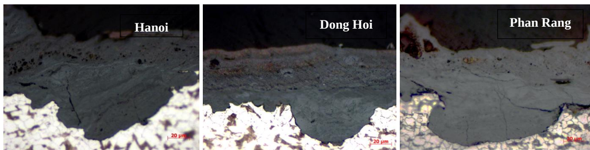
FIGURE 4. THE CROSS-SECTION OF RUST LAYER FORMED ON WS EXPOSED FOR TWO YEARS AT TEST SITES
