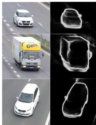
FIGURE 10: Examples of contour detection using the pre-trained model
