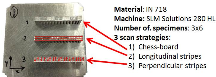
FIGURE 2: SCANNING STRATEGIES FOR THE MANUFACTURING OF CANTILEVER SPECIMENS IN ONE BASEPLATE. 6 EQUIVALENT BASE PLATES WERE MANUFACTURED IN THE SAME BATCH
