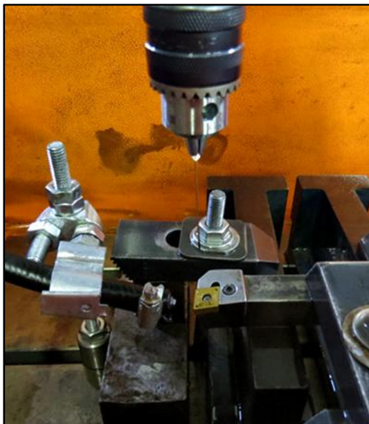
FIGURE 1: DRILLING OF INSERTS USING ELECTRICAL DISCHARGE MACHINING
