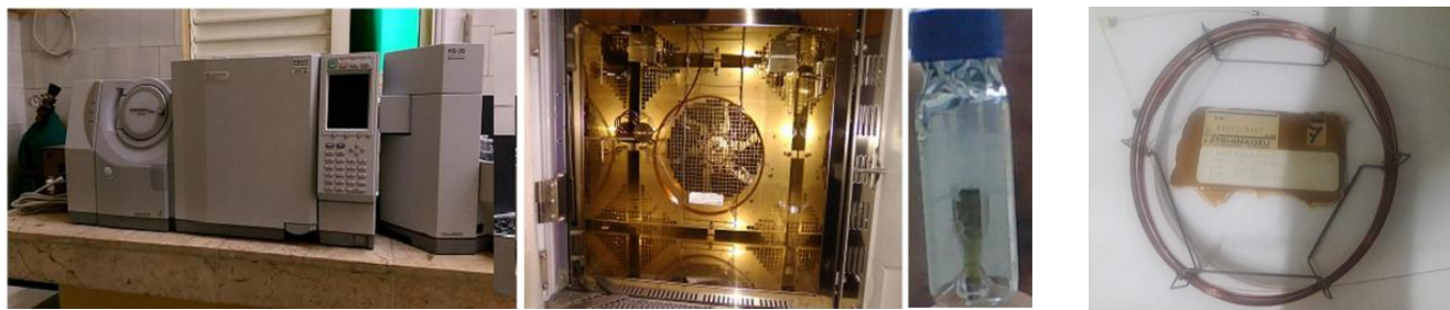
FIGURE 2: GC-MS Shimadzu QP2010, BP5 capillary column and derivatization process of the sample used in the experiment.
