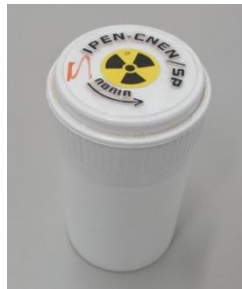
FIGURE 5: Shielding and storage device. Dimensions: 10 cm height and 5.2 cm diameter. Volume = 212.37 cm^3 .
