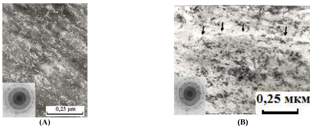
FIGURE 2: Formation of nanostructures at t = 0.9 \text{ ks} on the nickel surface at nominal contact pressure: a) 84 kPa; b) 168 kPa
