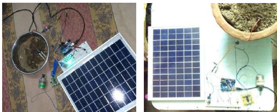
FIG 11. SNAPSHOTS OF AUTOMATIC SOIL MOISTURE MONITORING SYSTEM
