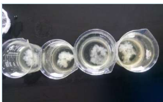
FIG. 5 SAMPLE PICTURES OF FRACTURE LIQUID AFTER BREAKING WITH DIFFERENT AMMONIUM PERSULPHATE LOADING OF 0.02 wt%, 0.03wt%, 0.04wt% and 0.05wt%, RESPECTIVELY.
