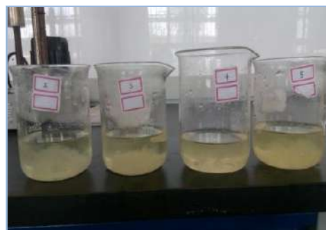
FIG. 5 SAMPLE PICTURES OF FRACTURE LIQUID AFTER BREAKING WITH DIFFERENT AMMONIUM PERSULPHATE LOADING OF 0.02 wt%, 0.03wt%, 0.04wt% and 0.05wt%, RESPECTIVELY.
