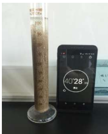
FIG. 1 SAND SETTLING TEST OF NEW NOVEL BORATE-CROSSLINKED GUAR GEL CONTAINED 20 WT% OF 20/40 SAND AT ROOM TEMPERATURE. A 0.3WT% GUAR LOADING IN FRESH WATER WAS ADDED INTO 0.4ML NaOH (10%) AND CROSSLINKED WITH 0.4 ML NOVEL CROSSLINKER.
