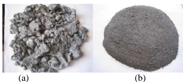
FIGURE 1. Sample of aluminum dross before (a) and after grinding (b)
