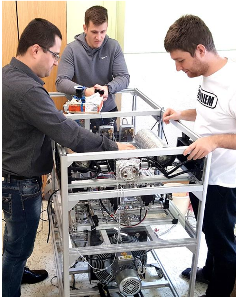
FIGURE 1: View of the final construction of the metal hydride compressor
