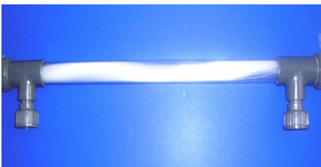
FIGURE 3: The bundle of fibres in a transparent tube
