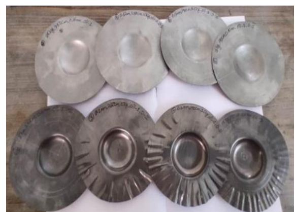
FIGURE 3: Deformed Superni 718work pieces
